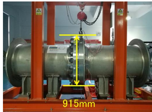
Fig. 1 Test equipment for bolted gasketed pipe flange connections (JPI Class300 4inch)
